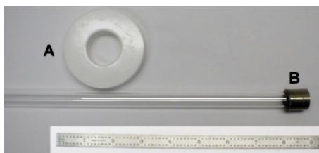
FIG. 3. Digital photo of: (A) plastic coated ferrite ring magnet, and (B) three 3/4 in. diameter, 1/2 in. thick cylindrical samarium cobalt magnets. The first is epoxied to the 0.5 in. diameter quartz transfer rod, and the other two magnets are stuck together by the magnetic force.
