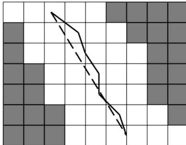
Fig. 6. Schematic (pixelated) representation of the nanowire (NW) fragment. Bright pixels represent the NW, and dark pixels are the background. Binning of pixels results in a representation (dashed line) that can be compared with the medial axis representation (solid curve) based on the use of all the bright pixels.
