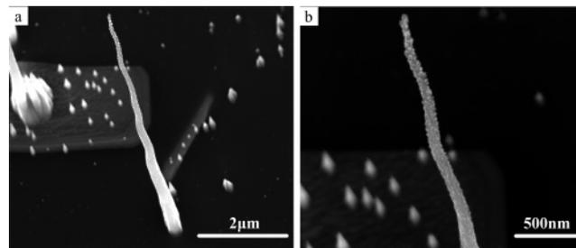
**Figure 5.** (a) SEM image of an isolated vertically aligned MWCNT coated with Ag nanocrystals, and (b) the enlarged view of the same MWCNT showing variations of the nanocrystal size and areal density along the length of the CNT.
