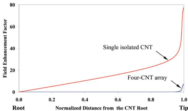
**Figure 6.** Electric-field-enhancement factor along the length of the CNT for a single isolated, vertically aligned CNT, and a four-tube square array with intertube spacing of 500 nm. The CNTs are 10  $\mu\text{m}$  in length and 150 nm in diameter. The spacing between the CNT substrate and the counter electrode is 2 mm.
