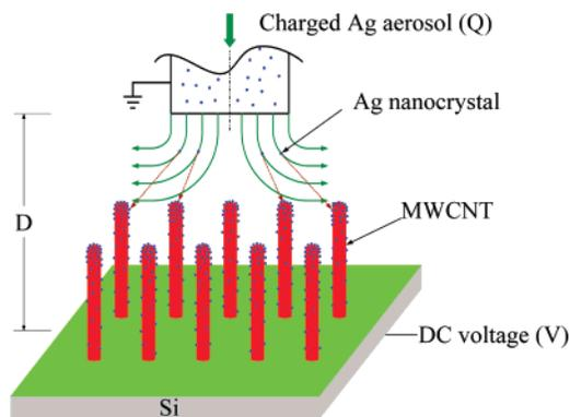
**Figure 1.** Schematic diagram for the assembly of Ag nanocrystals onto vertically aligned MWCNTs.
