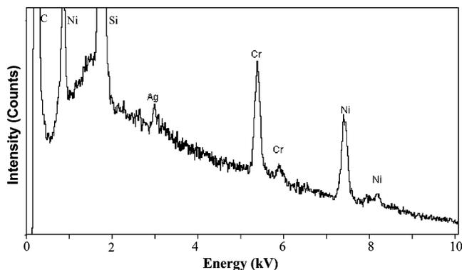
**Figure 3.** SEM-EDX spectrum of vertically aligned MWCNTs coated with Ag nanocrystals.
