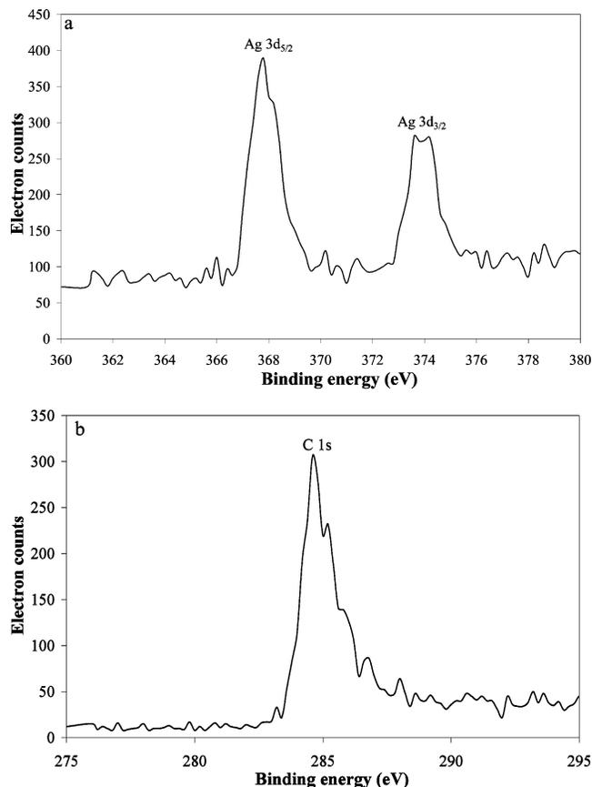
**Figure 4.** XPS spectra of (a) Ag 3d core levels and (b) C 1s core level of the aligned CNT array coated with Ag nanocrystals.
