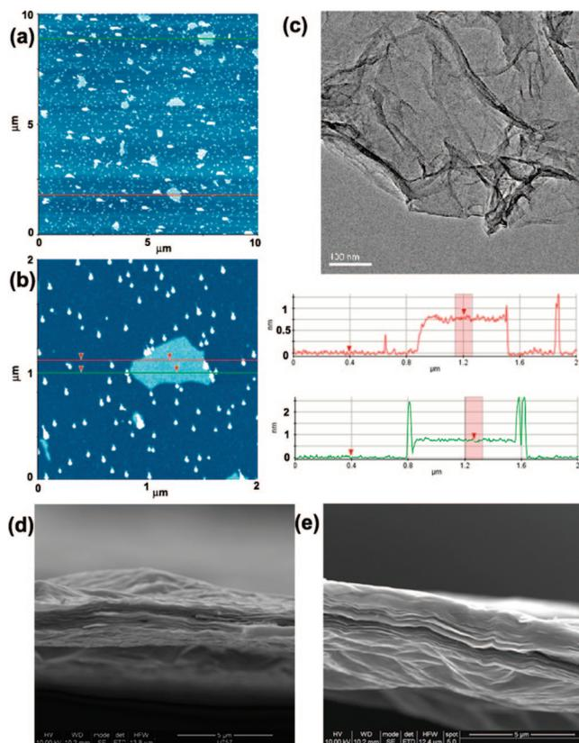
**Figure 2.** Microscopic images for HRG sheets. (a) An AFM image with 10  $\mu\text{m}$  scale, (b) an AFM image with 2  $\mu\text{m}$  scale, and (c) a TEM image, scale bar = 100 nm; SEM images of the cross-section of (d) the air-dried HRG paper and (e) the HRG paper that had been “dried” at 150  $^{\circ}\text{C}$  under Ar(g).
