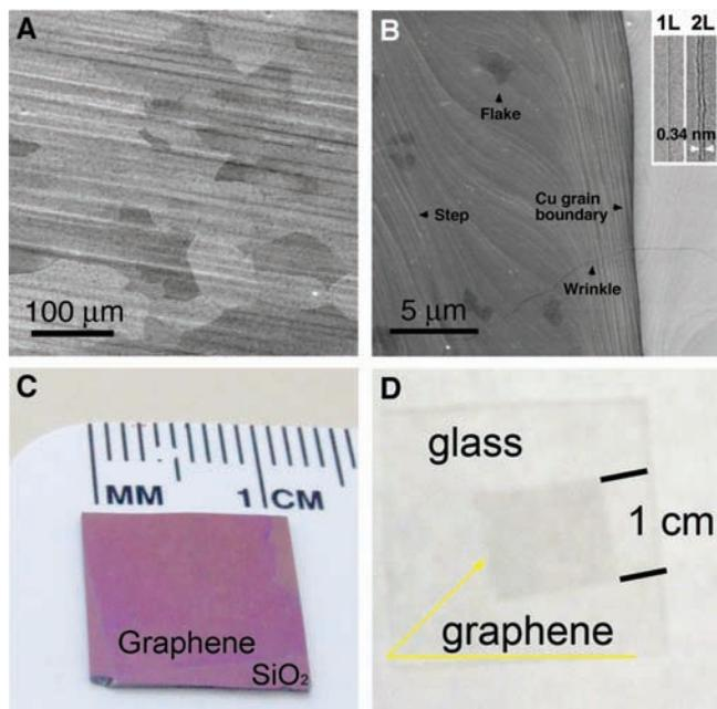
**Fig. 1.** (A) SEM image of graphene on a copper foil with a growth time of 30 min. (B) High-resolution SEM image showing a Cu grain boundary and steps, two- and three-layer graphene flakes, and graphene wrinkles. Inset in (B) shows TEM images of folded graphene edges. 1L, one layer; 2L, two layers. (C and D) Graphene films transferred onto a SiO<sub>2</sub>/Si substrate and a glass plate, respectively.
