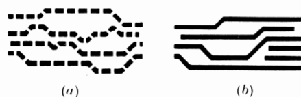
FIG. 4. Schematic representation of the structures of agglomerated G.O. soot and G.O. reduction product.
