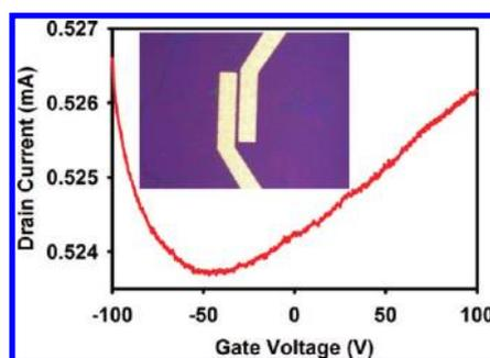
Figure 5.  $I-V_g$  curve of a field-effect transistor of HEFG film. The measurement was carried out in vacuum and bias voltage between source and drain electrodes was 0.1 V. The inset is an optical microscopy image of the device with the channel length of 4 μm.
