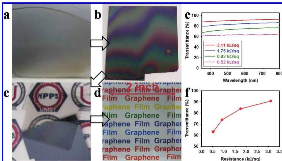
Figure 4. (a) Photograph of HEFG film on SiO<sub>2</sub> surface; (b) photograph of PMMA spin-coated on HEFG (HEFG/PMMA) film by spin coating; (c) freestanding HEFG/PMMA after SiO<sub>2</sub> surface etching; (d) 2 in. by 2 in. HEFG on PET (HEFG/PET) film; (e) optical transmittance with respect to wavelength; (f) transmittance vs sheet resistance curve.
