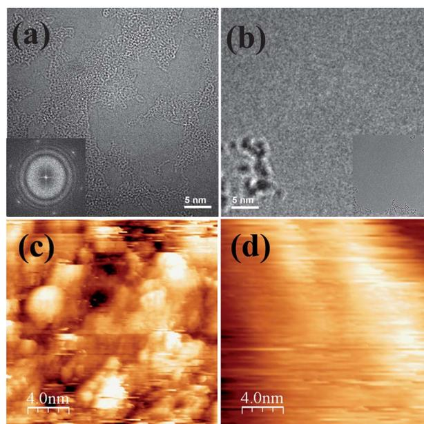
**Fig. 1** TEM images of suspended graphene (a) before annealing with FFT shown in the inset; (b) after annealing at 550 °C for a few hours, a low magnification image shown in the inset (700 nm<sup>2</sup> frame); STM images (c) before annealing and (d) after annealing at 550 °C. All images represent raw data. The STM scanning conditions were: tunnelling voltage of 0.5–1.5 V, current 0.1–1 nA.
