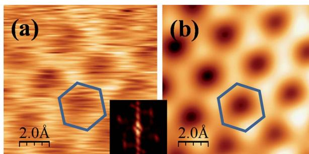
**Fig. 2** High resolution STM images of monolayer graphene. (a) Raw and (b) FFT filtered image. A hexagonal monolayer structure can be observed in both images. The image acquisition parameters were:  $V_{\text{bias}} = +0.6$  V and  $I = 0.3$  nA. The inset shows the FFT.
