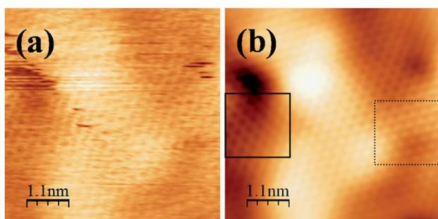
**Fig. 3** High resolution monolayer and bilayer graphene region. (a) Raw and (b) FFT filtered images. Hexagonal monolayer (solid line square) and triangular bilayer (dotted line square) structures can be observed in both images. The image acquisition parameters were:  $V_{\text{bias}} = +0.6$  V and  $I = 0.5$  nA.
