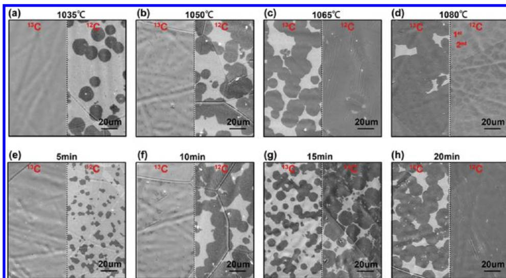
Figure 2. (a–d) SEM images of the <sup>13</sup>C (left panel) and <sup>12</sup>C-graphene (right panel) on Cu–Ni alloy foils for a deposition time of 10 min and different deposition temperatures. (e–h) SEM images of the <sup>13</sup>C-graphene (left panel) and <sup>12</sup>C-graphene (right panel) on Cu–Ni alloy foils for a deposition temperature of 1050 °C and various exposure times.
