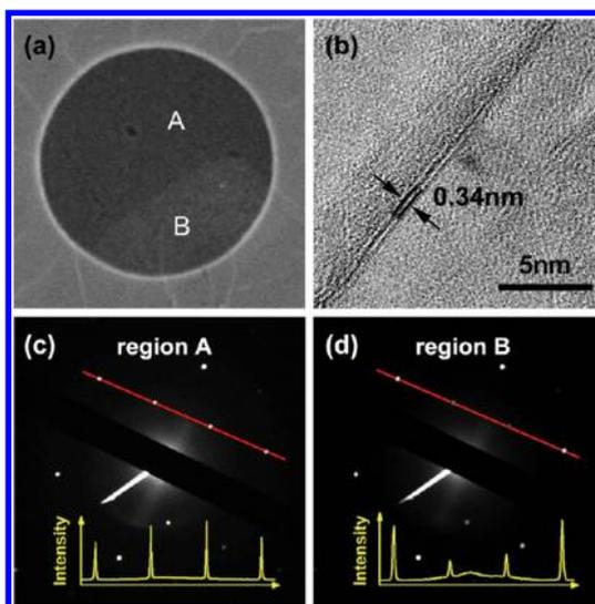
**Figure 6.** (a) SEM image of a graphene film transferred onto a TEM grid, with monolayer graphene in region A and bilayer graphene in region B. (b) high resolution TEM image taken in region B, with the distinct fingerprints showing an interlayer spacing of about 0.34 nm. (c and d) The SAED patterns and the corresponding intensities along the red lines measured in region A and B, respectively, implying monolayer and AB-stacked bilayer graphene.
