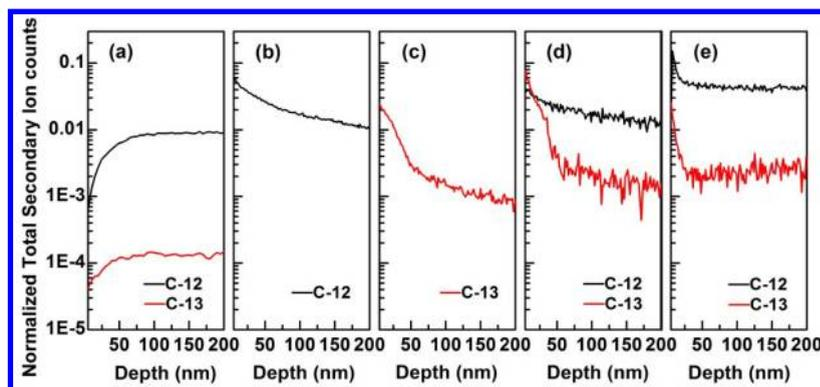
Figure 4. (a) The depth profiles of background  $^{12}\text{C}$  and  $^{13}\text{C}$  in Cu–Ni alloy foil without carbon deposition. (b,c) The depth profiles of  $^{12}\text{C}$  and  $^{13}\text{C}$  in Cu–Ni alloy foil for the two samples grown with only  $^{12}\text{C}$  or only  $^{13}\text{C}$  deposition, respectively. (d,e) The depth profiles of  $^{12}\text{C}$  and  $^{13}\text{C}$  in Cu–Ni alloy foil for the two samples with opposite isotope-deposition orders.
