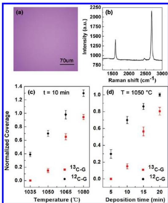
**Figure 3.** (a,b) Optical microscope image and a typical Raman spectrum taken from monolayer graphene transferred onto a 285 nm SiO<sub>2</sub>/Si substrate; (c,d) Normalized temperature-dependent and carbon-deposition-time-dependent coverage of <sup>12</sup>C- and <sup>13</sup>C-graphene, respectively. The error bars are generated by examining some SEM images at each growth condition.
