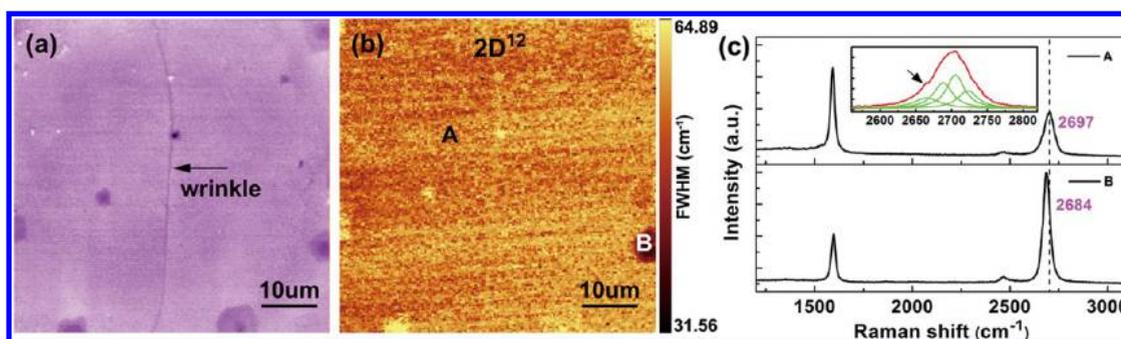
Figure 5. (a) Optical microscope image of bilayer graphene transferred onto a 285 nm  $\text{SiO}_2/\text{Si}$  substrate. (b) Raman map of the fwhm of  $^{12}\text{C}$ -2D ( $2\text{D}^{12}$ ,  $2650\text{--}2750\text{ cm}^{-1}$ ) band from the same area in panel a. (c) Raman spectra from the positions marked by A and B in panel b.
